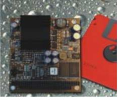
PC/104 bus products. The flash SSD emulates a standard FDD, a complete PC system can thus be assembled from just one Micronix PV-5124 and one PC/104 CPU.
